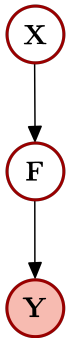
Figure 3.4: Graphical model for GPLVM. Y is observed and the map F and the input X are latent.
