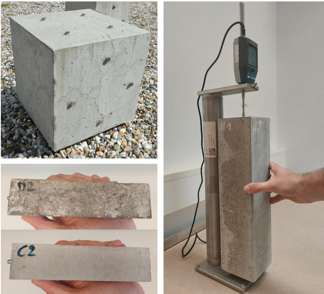
Figure 22: Photographs of specimens from ASR expansion tests. Top-left: cracked 30 cm field cube with PC-HA. Bottom-left: TI-B 51 mortar bars after 20 weeks of exposure. Right: length measurement of an AAR-10 concrete prism.
