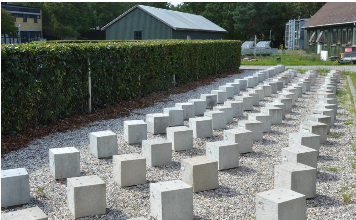
Figure 9: ASR field exposure site at DTU, established in 2017 (GPS coordinates: 55.79103, 12.52619). In total, 90 cubes are currently exposed to test different aspects such as the aggregate type, the binder type or the effect of impregnation.
