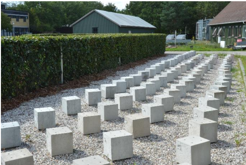
Figure 1: Field exposure site at the Technical University of Denmark (Kgs. Lyngby, Denmark).
