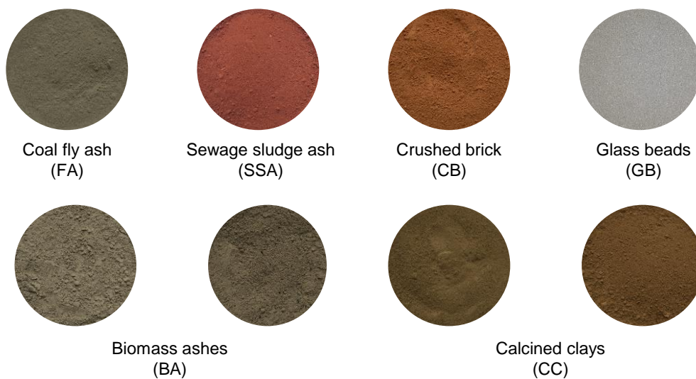
Figure 7: SCMs investigated in the project. A limestone filler was also included in paste experiments, as a reference inert material.
