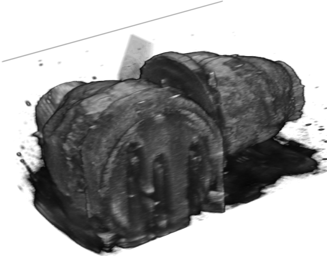
Figure 7.3: Volume rendering from a series of B-mode scans in the sliding fixture. See (Garreau 2019). This data were acquired using a convex probe with an output pixel size of (0.15 mm, 0.15 mm) and an inter slice distance of 2 mm.
