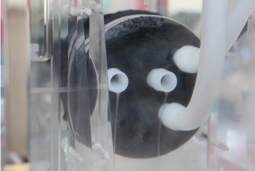
Figure 4.2: DHP inlet/outlet connectors. Tubes are connected to the LV, pumping BMF. The BMF leaking from the RV is caused by a defect in the phantom.
