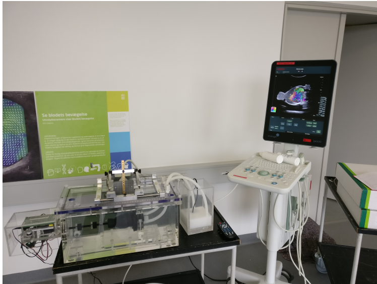
Figure 7.4: Example of setup for VFI acquisition. The scanner monitor provides a live preview of the flow direction and magnitude as an overlay to a B-mode image. Note the fluid in the fluid reservoir is milky white. This is the blood mimicking fluid which is necessary for performing VFI measurements.
