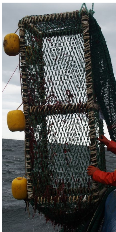
Figure 5.1.1: Picture of the constructed codend with fixed meshes.
