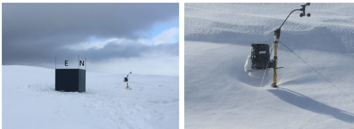
Fig. 3. Cube and nearby weather station with wireless data transfer to receiver and logging computer. The distance between cube and station is 3m.
