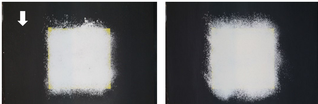
1. Baking powder U_{Th,Pitot} = 10,26 [m/s] 2. Flour (Wheat) U_{Th,Pitot} = 10,34 [m/s]
