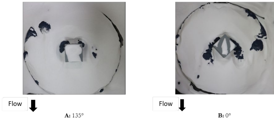
Figure 9 A photograph of the model Nuuk cube in scale 1:20 during test performance. A: First snowfall and erosion test: Snow accumulation with flow direction from Southeast 135° B: Second snowfall and erosion test: Snow accumulation after flow direction from North 0°.
