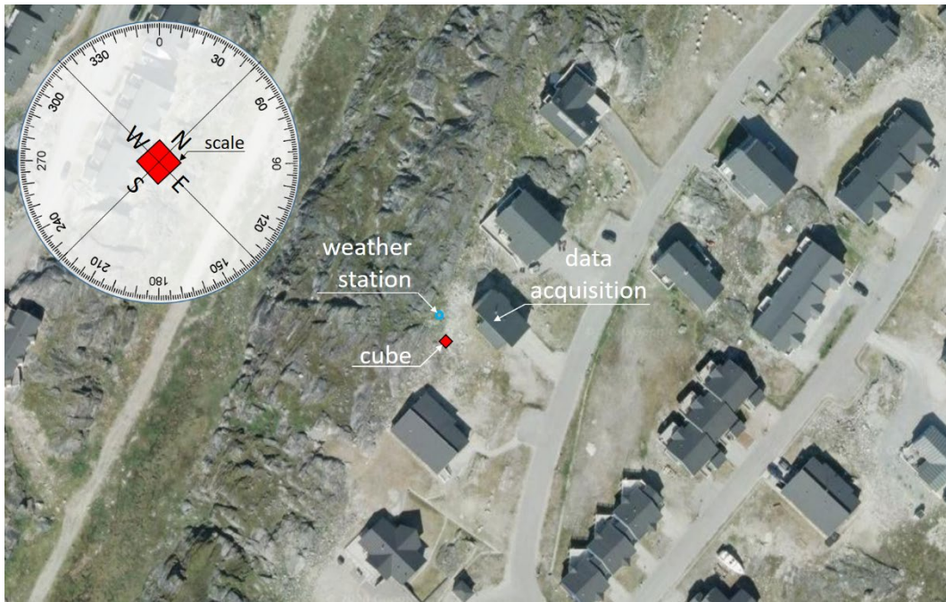
Fig. 2. The cube has been installed on an open stretch 13m west of the nearest building (observation base, housing of data acquisition computer). The surface topography is moderately uneven but still flat enough to allow representative snowdrift and accumulation. The footprint of the cube is rotated 45° to north south direction to face the most frequent direction for snow events based on experience (Google Earth, accessed on October 9, 2020). Geographic reference of cube position 64°11'37.3"N 51°42'121.2"W (64.1936, -51.7030), elevation 36.7m above sea level (position and elevation provided by land registry office for Nuuk).
