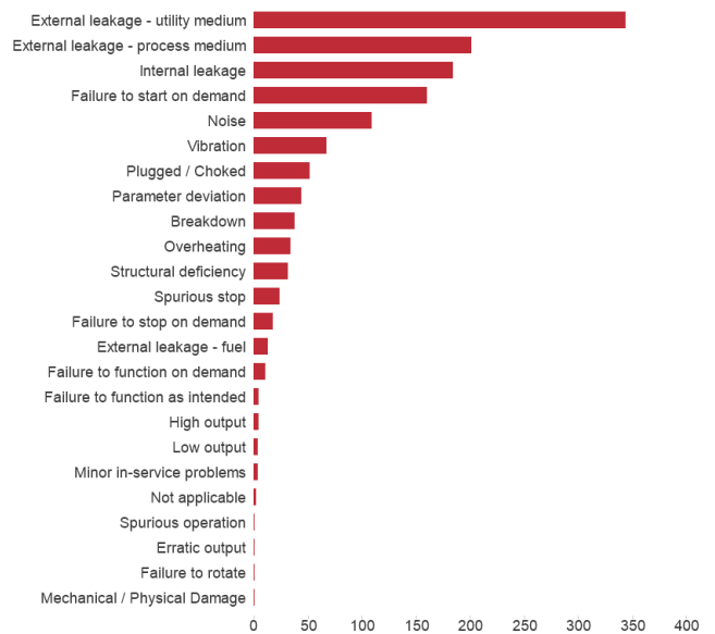
Fig. 5. The distribution of pump failures across failure modes at the case company.
