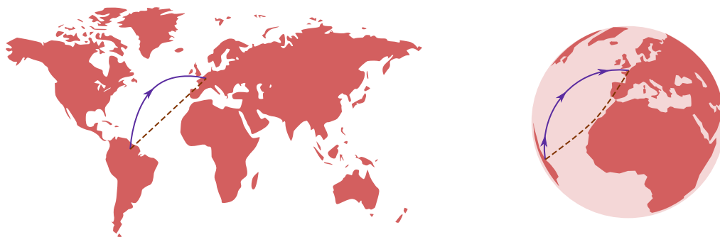
Figure 1.1: The shortest path between Cayenne and Paris is not a straight line on the map.
