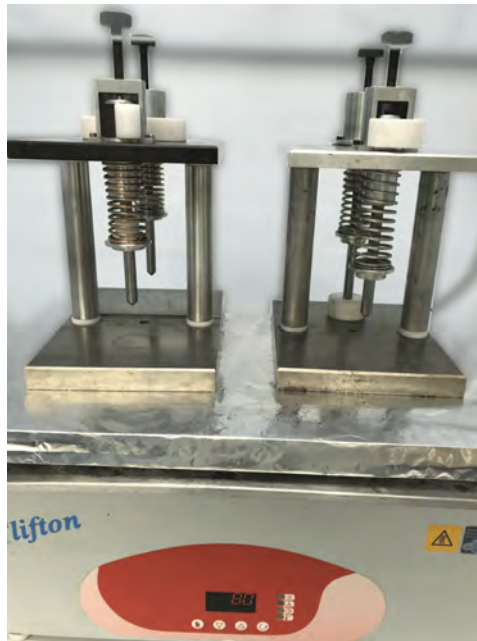
Figure 4.10: Image of two bonding jig stations used to mount the wafer onto a glass substrate prior to lapping. The bonding station is placed on top of a hot plate.
