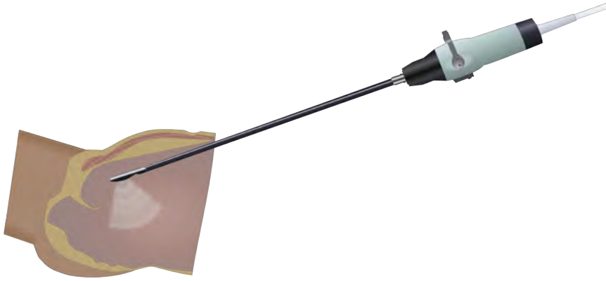
Figure 1.6: Conceptual overview of a laparoscope with an integrated ultrasound transducer used for guidance during surgery in the abdomen.
