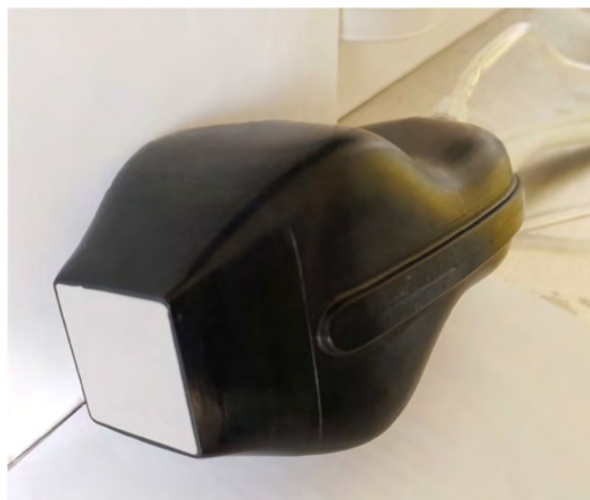
FIGURE 9. Assembled three-part custom 3D milled PPSU probe handle. The RCA CMUT array is buried underneath the stack of RTV silicone, aluminium polymer foil and silicone covering the nose piece. The two cooling hoses can be seen protruding beside the scanner cables.
