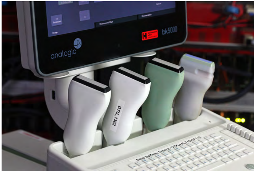
Figure 1.4: Four CMUT-based linear probes designed and fabricated by Ph.D. Søren E. Diedrichsen [16].
