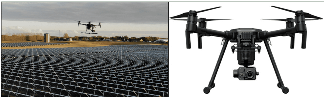
Figure 2.13: DJI Matrice 200 equipped with a Zenmuse XT2 camera flying over the solar collector field in Vojens (left) and close-up photo (right) (Drones Made Easy, n.d.).
