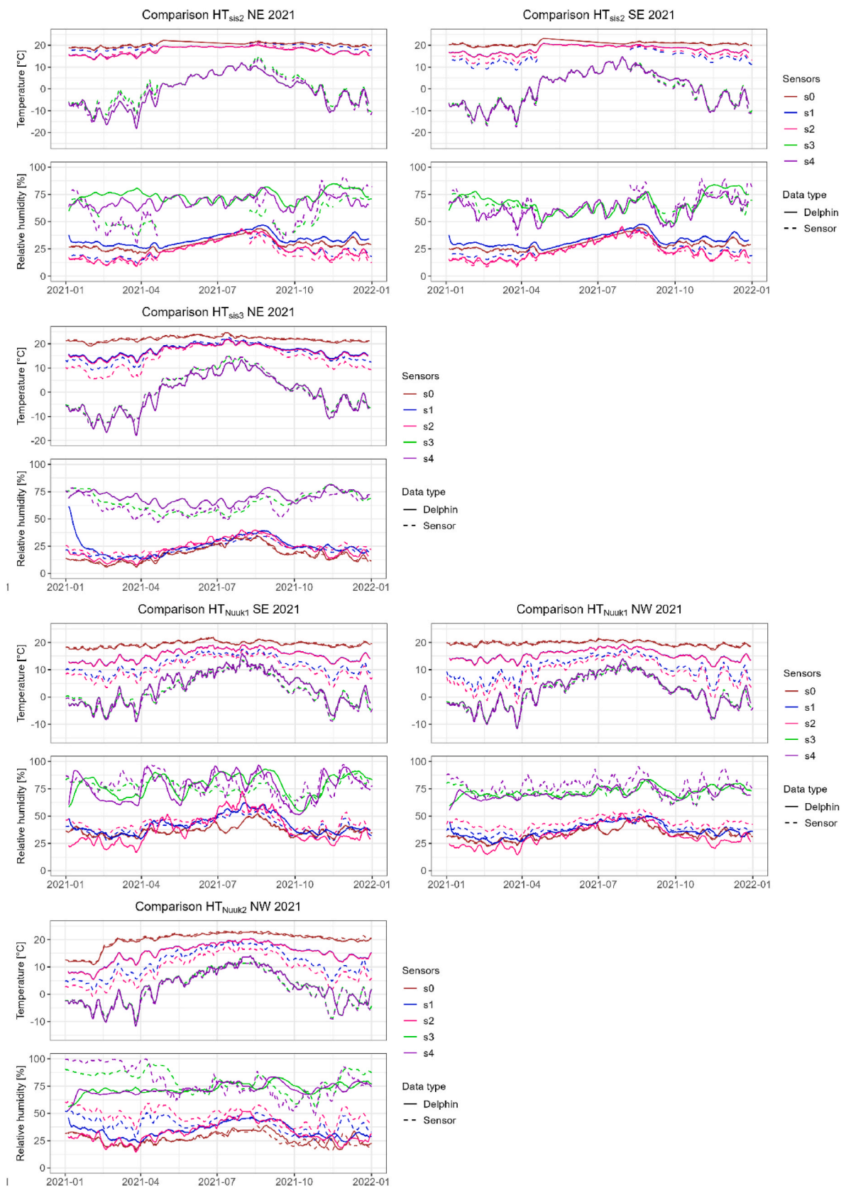
Fig. 5. Comparison of the measured hygrothermal conditions and the results of Delphin models for selected houses, orientations, and years. All graphs are displayed for moving mean values of 7 days.
