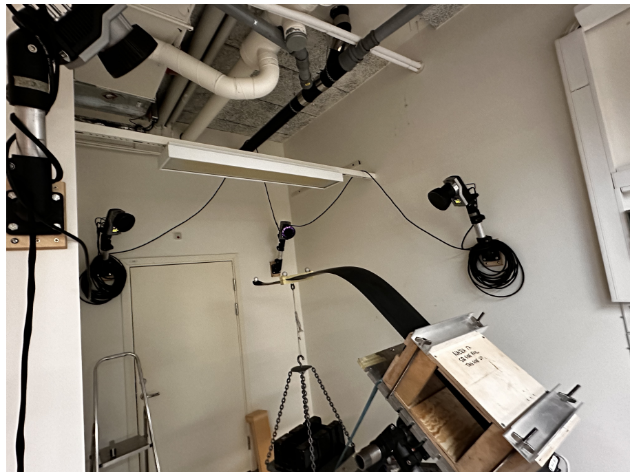
Figure 11. Rig used to test the structural twist and deformation of a NACRA 17 foil.
