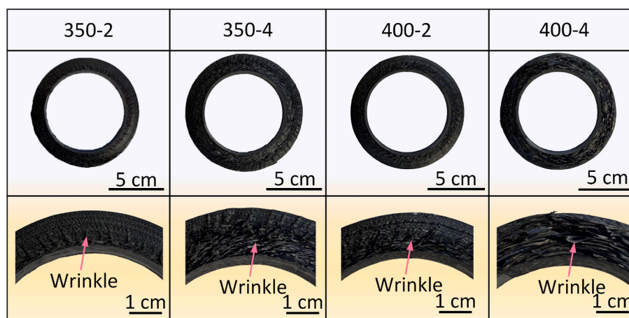
Fig. 6. Macro-appearance of specimens manufactured by different parameters. The second row magnified images show the presence of wrinkles.
