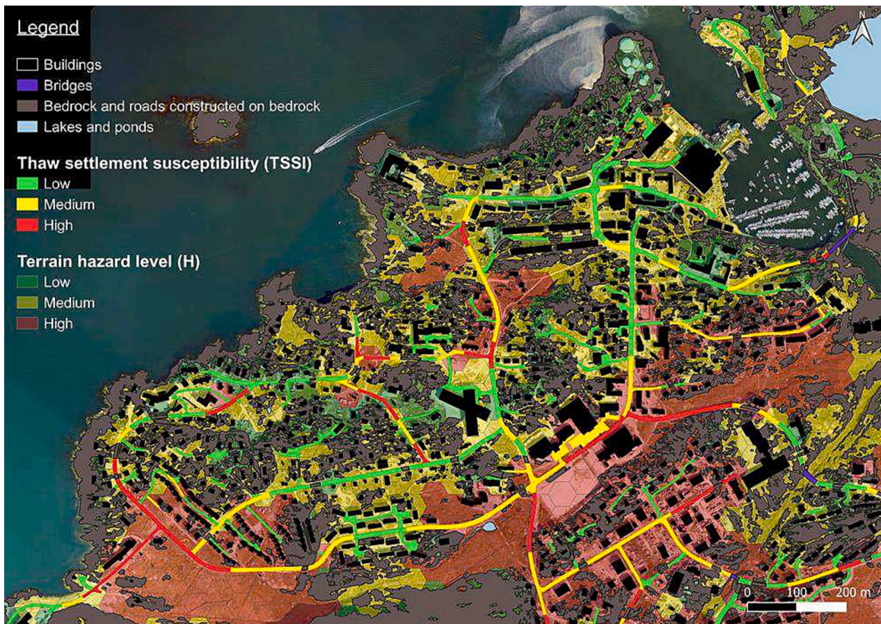
Fig. 10. Thaw settlement susceptibility map (2012–2021) of Ilulissat's road network. The map contains an orthophoto and spatial data from Asiaq, Greenland Survey, Basemap, 2022 (Asiaq Greenland Survey, 2022).
