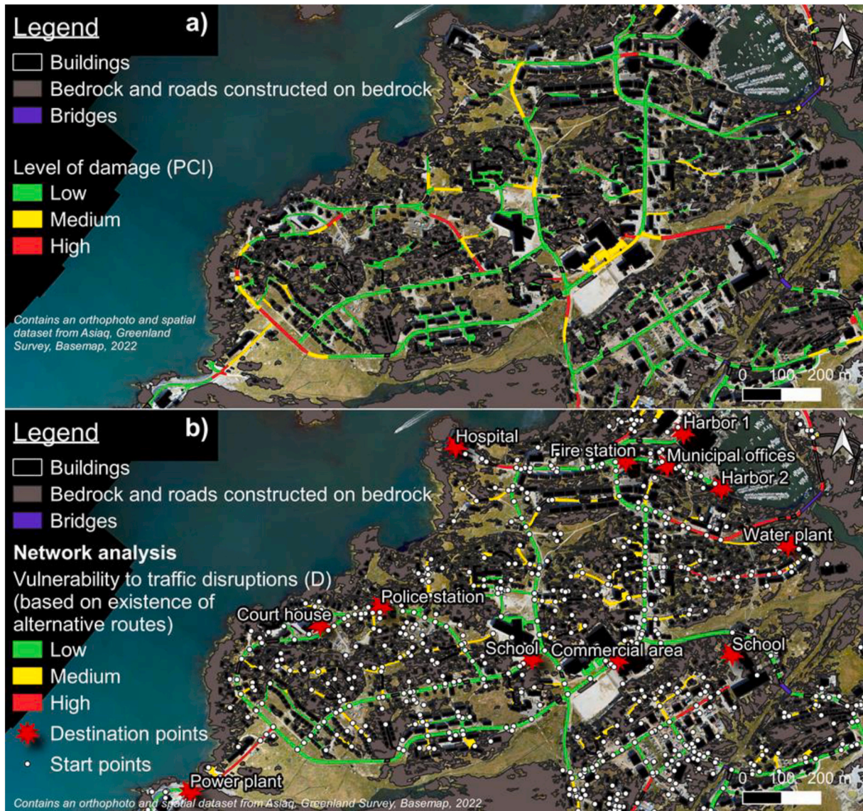
Fig. C.12. From top to bottom: (a) Road level of damage assessed with the Pavement Condition Index (PCI) (ASTM International, 2008), and (b) vulnerability to traffic disruptions (D). The maps contain an orthophoto and spatial data from Asiaq, Greenland Survey, Basemap, 2022 (Asiaq Greenland Survey, 2022).
