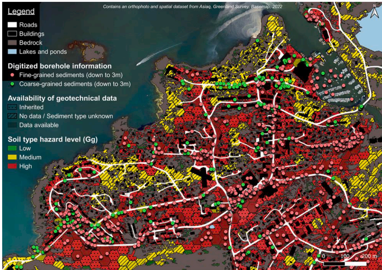
Fig. A.11. Borehole information used to assess the soil type hazard levels, G_g , across the study area. The green and red dots show the borehole classification based on the presence/absence of fine-grained sediments down to 3 m below the ground surface. The patterns overlaid onto the hexagonal terrain unit represent the availability of the geotechnical data. The map contains an orthophoto and spatial data from Asiaq, Greenland Survey, Basemap, 2022 (Asiaq Greenland Survey, 2022).
