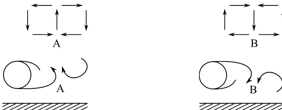
(a) Vortex shedding from lower side of cylinder. Ejection of particles at point A.
