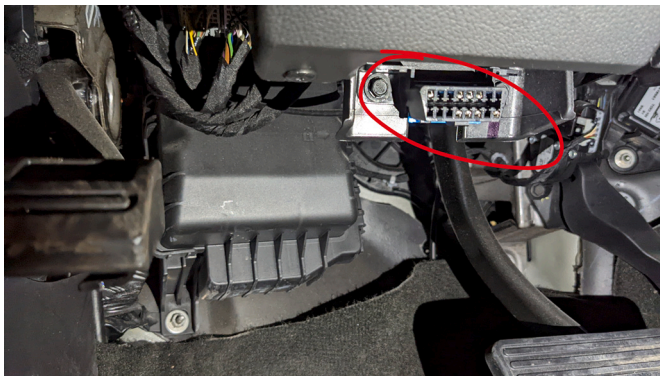
Fig. 11. The OBD-II port (Falch, 2022) of a 2016 Chevrolet Silverado. We accessed this port—via Korlan USB2CAN (8devices, 2023)—in order to capture CAN traffic and conduct attacks.
