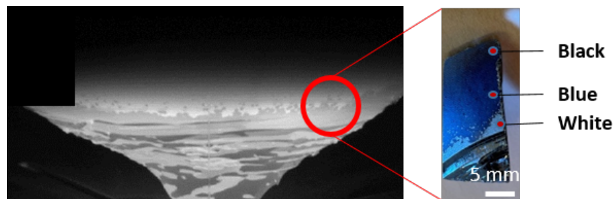
Figure 2.2: Comparison between an FZ image with a visible surface anomaly on polysilicon and the corresponding polysilicon part obtained from a terminated process.
