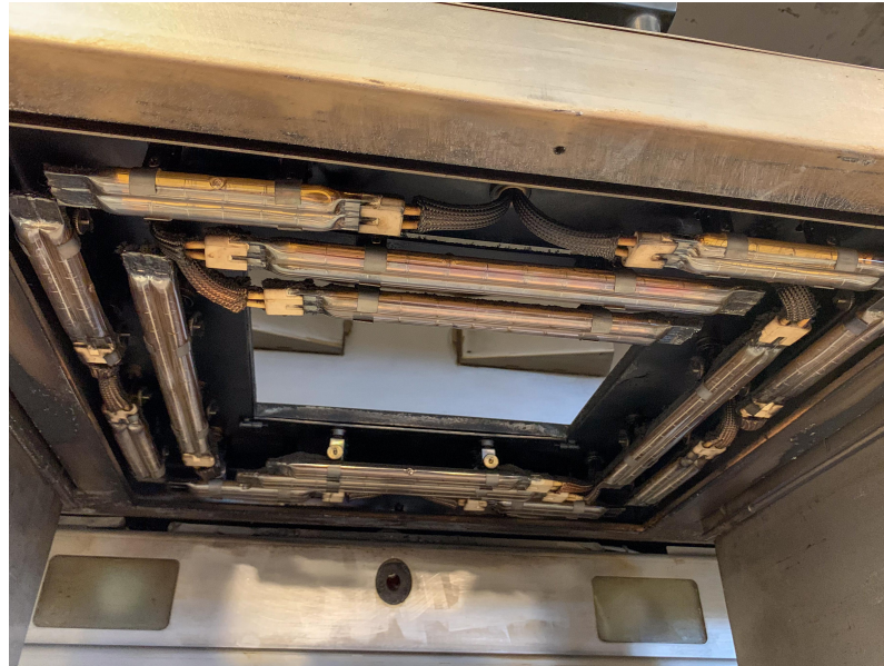
Figure 4.21: Double quartz lamp top heater array on the SinterStation 2000 in the AMIST centre at the University of Louisville
