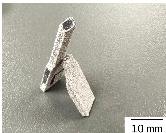
Figure 7.13: Cross-section view of a part produced from the 95-5 batch
