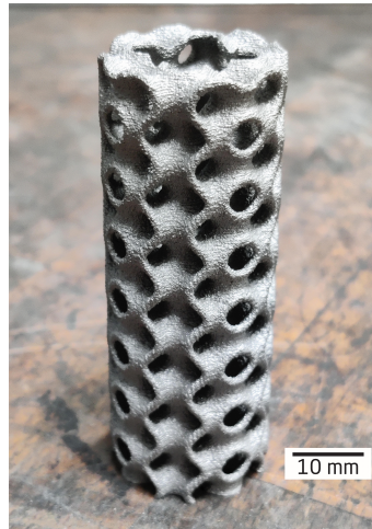
(c) Part with no post-processing
