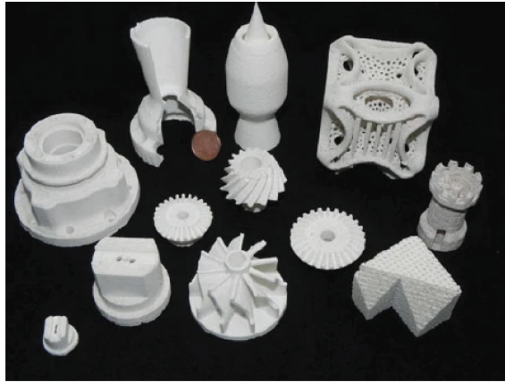
Figure 2.8: Showcase parts manufactured from ceramic Alumina powder. From Juste E. et al. [60]
