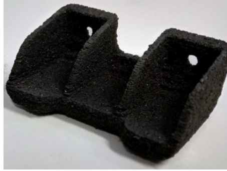
Figure 2.9: Composite bracket developed by NASA for high-temperature capability. The composite includes Polyimide and short-strand carbon fibres. From [62]
