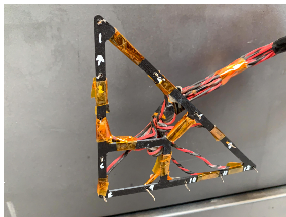
(c) K-type thermocouples integrated into the plastic sensor array
