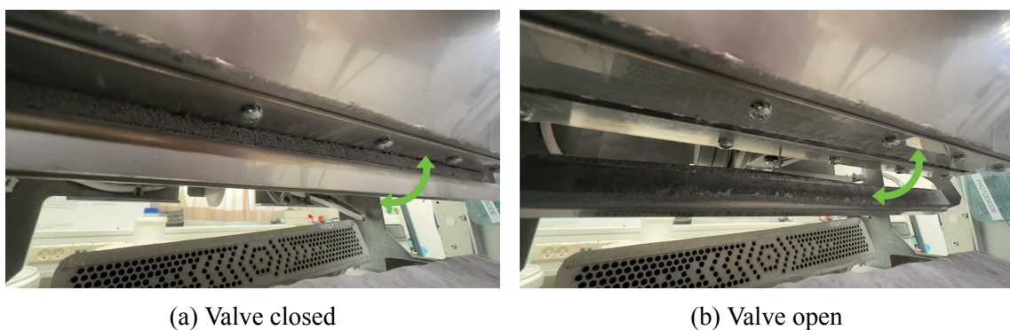
Figure 5.7: Dosing valve in the bottom of the hopper for not over-dosing powder
