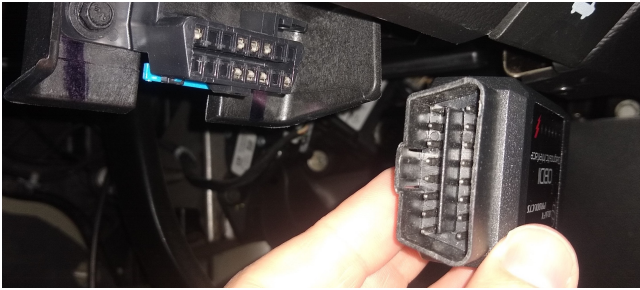
Figure 3: The on-board diagnostic port (left) and a diagnostic device (right).
