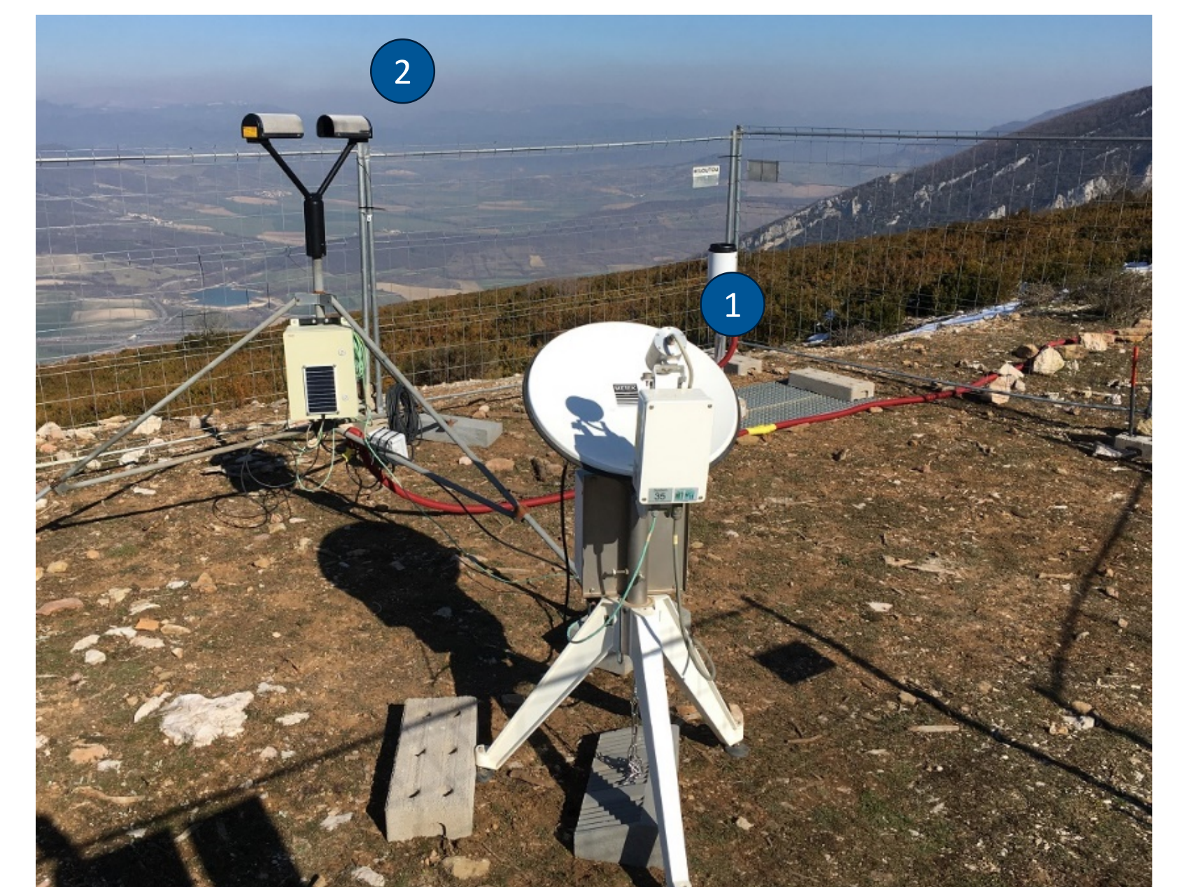
Figure 3. ALAIZ site with micro rain radar (1) and disdrometer (2).
