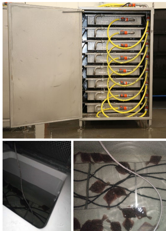
Figure 23. Survival unit to hold fish onboard the vessel (top) and transportation tank to the holding facility with oxygen supply (left and right).
