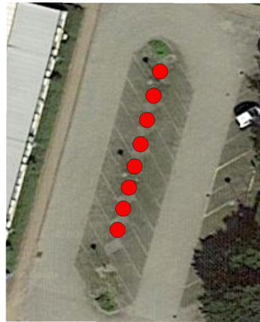
Fig. 3. Satellite picture of the parking lot location. The red dots indicate the chargers.
