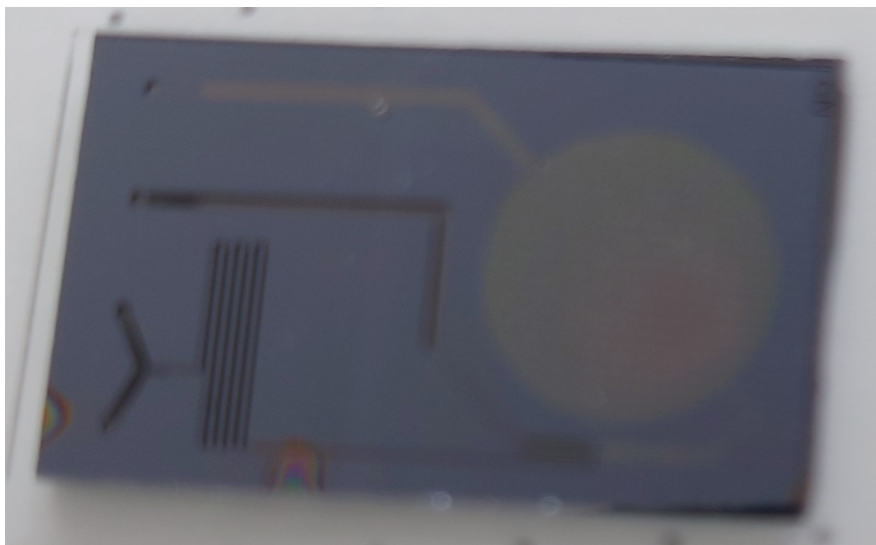
Figure 4.23: \mu -reactor with an incomplete bonding on the inlet gas side.
