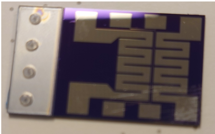
Figure 4.18: Image of a faulty bonded back spacer on a \mu -reactor.
