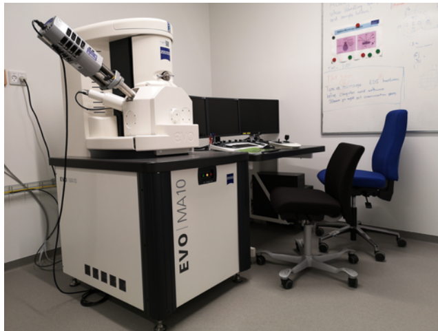
Figure 2.6. Zeiss EVO MA10 SEM with energy dispersive X-ray spectroscopy (EDS).
