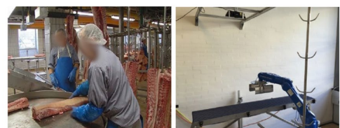
(a) Human involved meat pick and place process (b) Autonomous meat pick and place experimental setup
