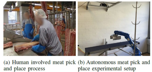
Fig.3 The illustration of the pick and place task in a slaughterhouse. (a) is the case when humans are involved in the task in the traditional process. (b) is the robotic algorithm testing hardware in the lab at DTU [9] .
