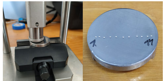
Fig. 3 Setup for IIT of PIIS 3000 (left) and results on SS304L sample (right)
