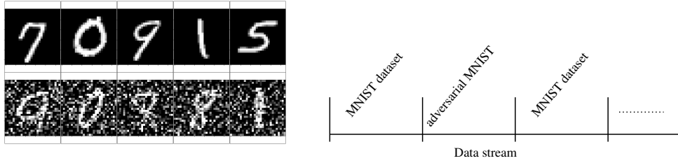
Figure 4: MNIST problem with adversarial samples: This example illustrates the transition between the sequence of images before and after the injected drift. The second row of images contains the sequence of adversarial samples.
