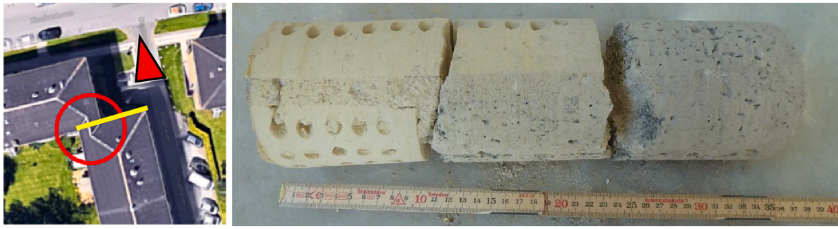
Fig. 3. Left: Top view of the building showing the covering of the neighboring property and the refurbished wall (yellow) [34] (Copyright Google Maps). Right: Drill core from original wall of case D. The outer part of the wall (on the left) is made of yellow brick and the inner part of lightweight clinker concrete (on the right). (For interpretation of the references to colour in this figure legend, the reader is referred to the web version of this article.)
