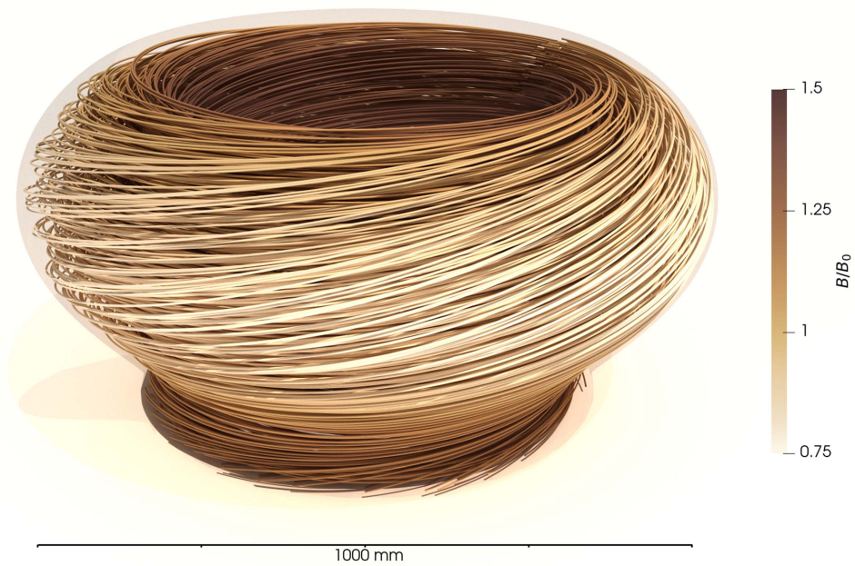
Figure 3. Streamlines of the magnetic field vector \mathbf{B} integrated and visualised in ParaView [71]. One low-opacity iso-contour of \rho_p = 1.10 is plotted (corresponding to \psi_p = 4 ). The positive \mathbf{B} direction is clockwise if viewed from above and the field-line winding is left-handed. \mathbf{B} \times \nabla B points towards the magnetic X-point and we have a favourable drift direction.
