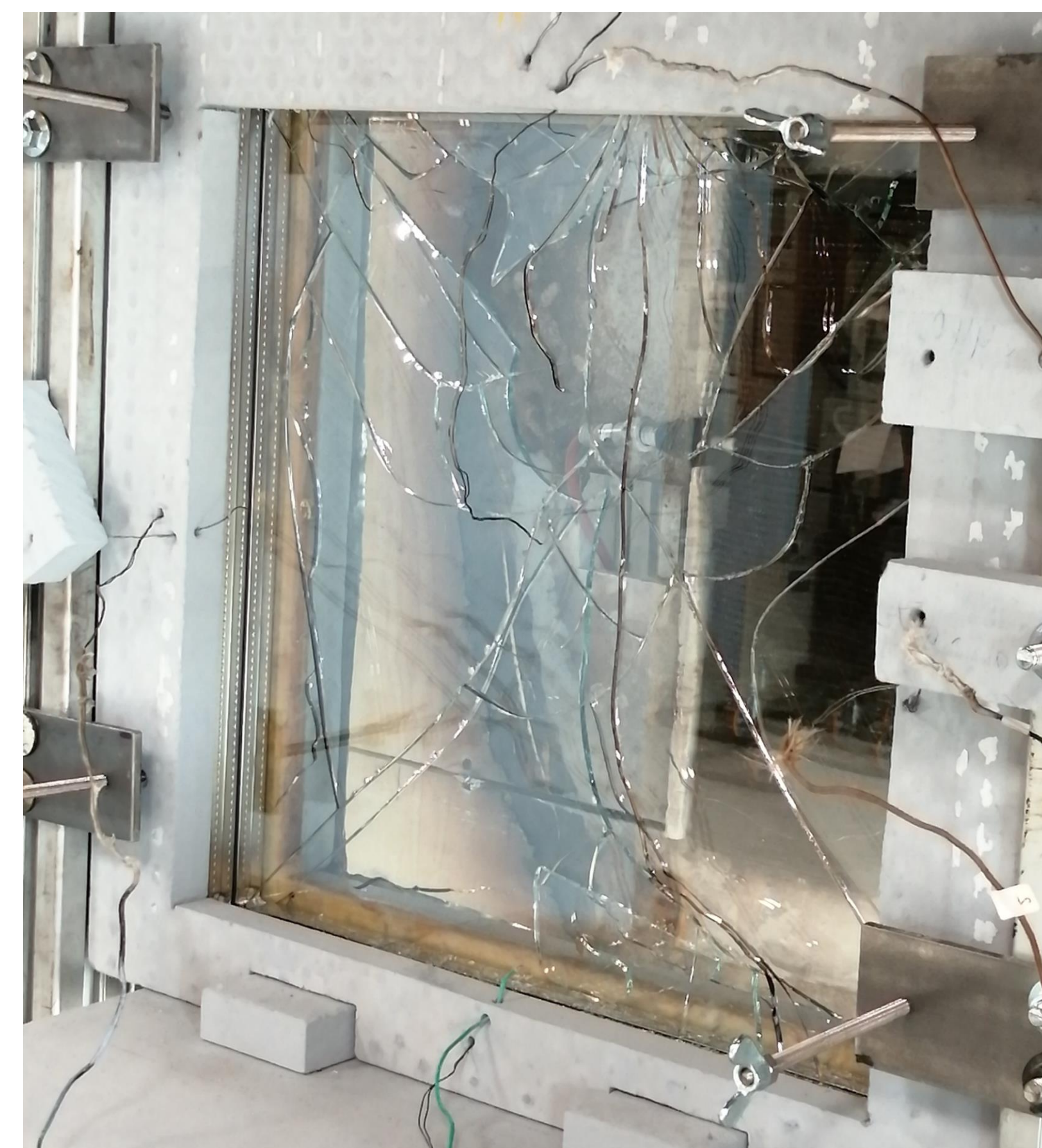
Fig. 1: Cracked glass panes after testing. Photo by Hvidberg [7].
