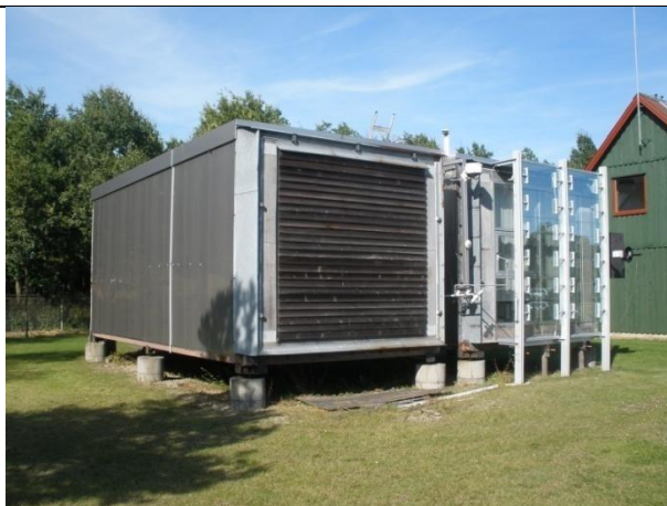
Outdoor test cells for test of hygrothermal room performance and test of daylight control systems
