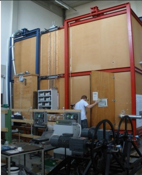
Cold and hot box chambers
