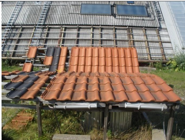
Outdoor test stand for weatherization test of roof tiles
