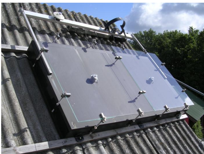
Figure 1. Test facility used to measure the solar transmittance of two glasses.
