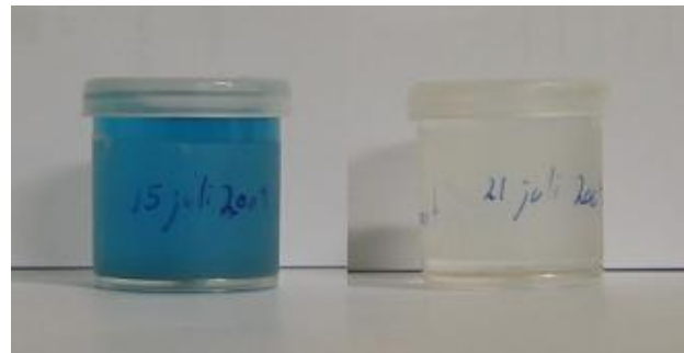
Fig. 5: Samples from the system extracted from the roof at the outlet of the collectors.
