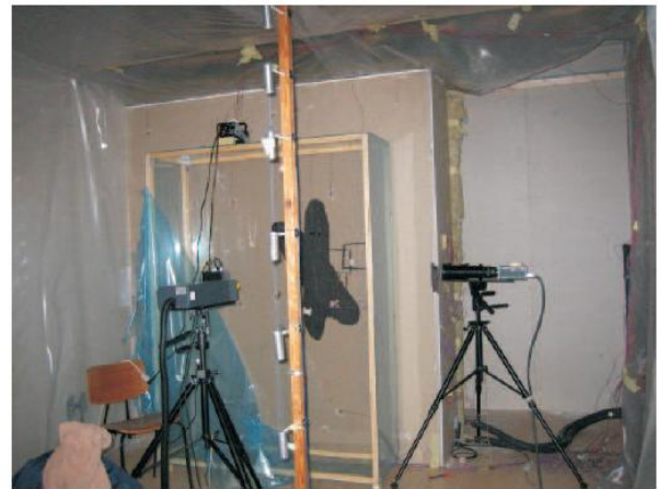
Sketches and a picture illustrating how PIV equipment was used to measure air velocity between a piece of (superficial) furniture and a cold wall.
