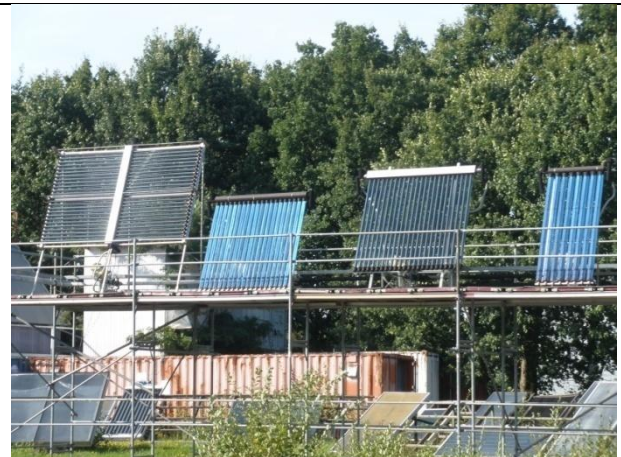
Test stand for vacuum tubular solar collectors
