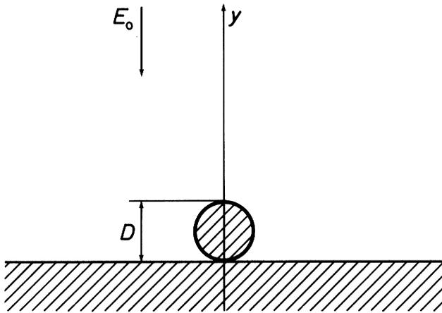
Fig. 1: Surface roughness model - circular wire.
