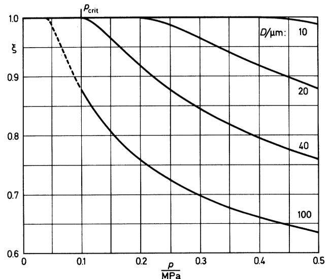
Fig. 2: Surface roughness factor  $\xi$  for  $\text{SF}_6$ .
