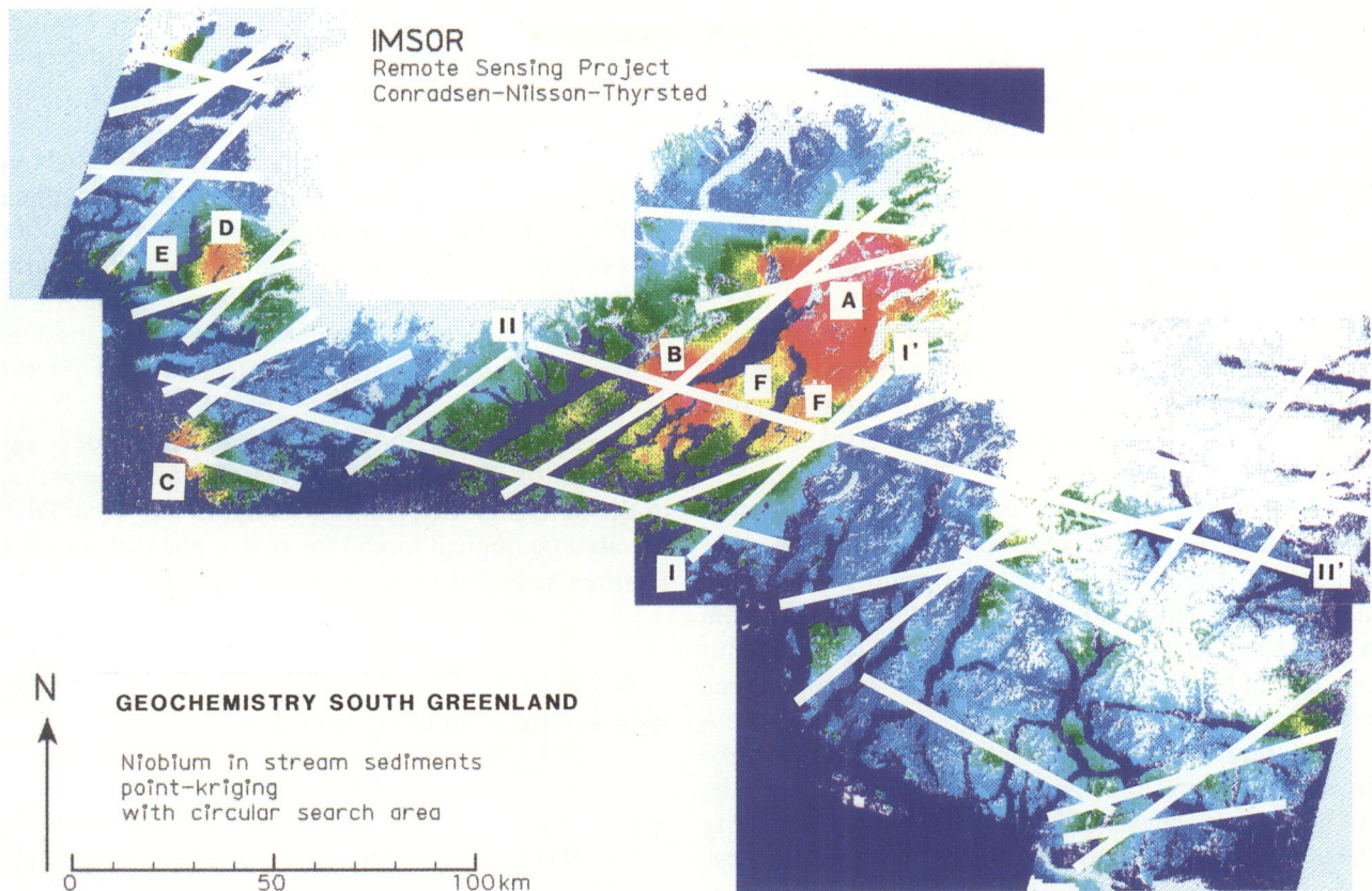
Fig. 7. Interpreted major lineaments superimposed on a niobium geochemical map with red, green, and blue colors indicating respectively high, intermediate, and low niobium content. Letters and roman numerals refer to localities mentioned in the text.
