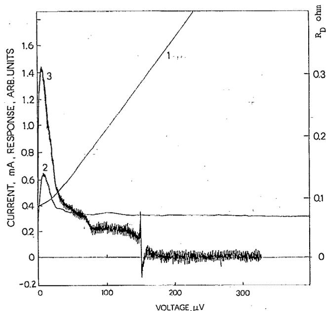
FIG. 1. (1) dc  $IV$ -characteristic, (2) voltage dependence of the differential resistance,  $R_D(V)$ , and (3) response  $\Delta V(V)$  to 73 GHz radiation for YBa<sub>2</sub>Cu<sub>3</sub>O<sub>7-x</sub> grain-boundary junction GBJ13. The temperature is  $T = 78 \text{ K}$ .
