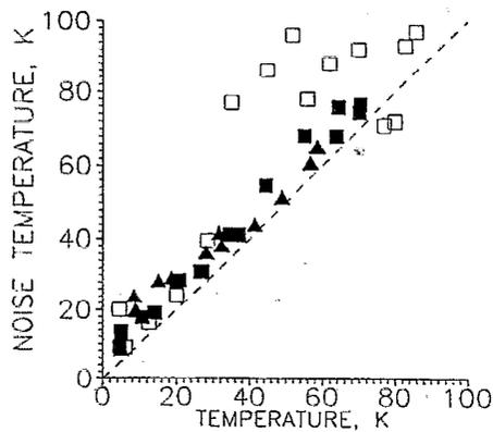
FIG. 3. Noise temperature vs physical temperature of the  $\text{YBa}_2\text{Cu}_3\text{O}_{7-x}$  grain-boundary junctions derived from the experimental values of the millimeter-wave Josephson linewidth. Filled triangles—GBJ21; filled squares—GBJ22; open squares—GBJ12.
