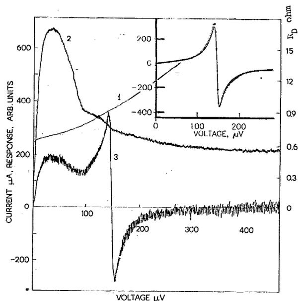
FIG. 2. (1) dc  $IV$  characteristic, (2) differential resistance, and (3) response to 72 GHz radiation for YBa<sub>2</sub>Cu<sub>3</sub>O<sub>7-x</sub> grain-boundary junction GBJ12 at  $T = 78 \text{ K}$ . The inset shows the normalized response  $h(V) = (\Delta V/R_D) I \cdot V$ , calculated and experimental.
