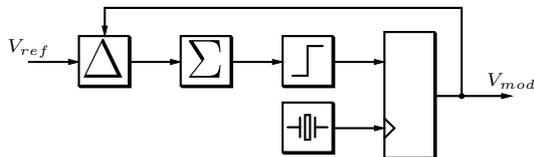
Fig. 4. Block diagram of a  $\Delta\Sigma$  modulator
