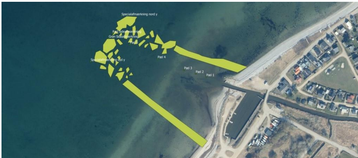
Figure 1 – Illustration of the established stone reef in front of River Storå. The yellow markings illustrate location of the stones. Fish migrating from the river and into the sea will encounter the reef (the yellow markings) and likely benefit from elevated shelter availability and extra food resources in the area.
