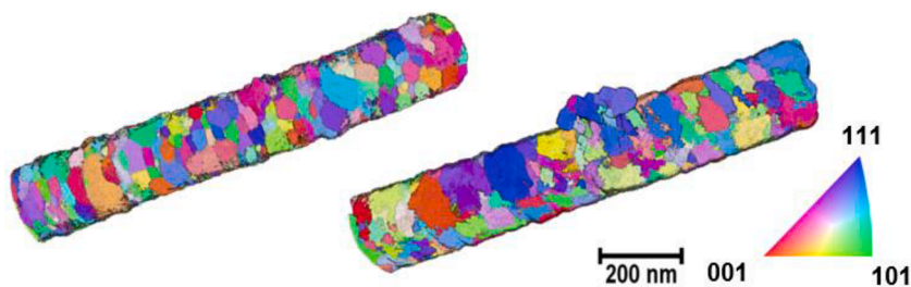
Fig. 1. Orientation maps of electrospun CGO fibre calcined at 800 °C. Left: calcined for 1 hour. Right: calcined for 10 h. The colours are inverse pole figure (IPF) colouring showing crystal directions.
