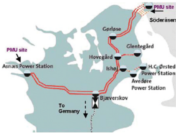
Fig. 2. 400-kV transmission grid in Eastern Denmark. One PMU was placed at ASV, and another PMU was placed 200 km away at SAN in Southern Sweden.
