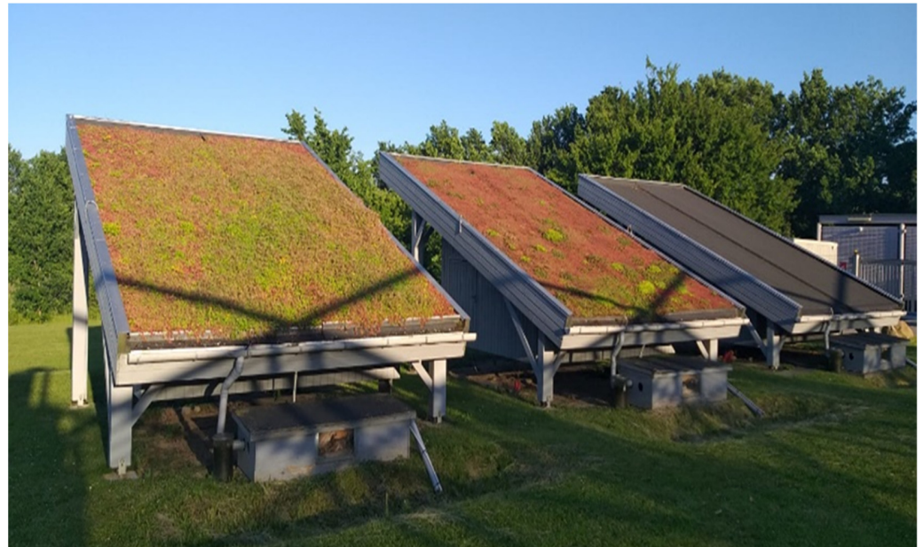
Figure 2. Overview of the three roof pilots used as experimental apparatus.
