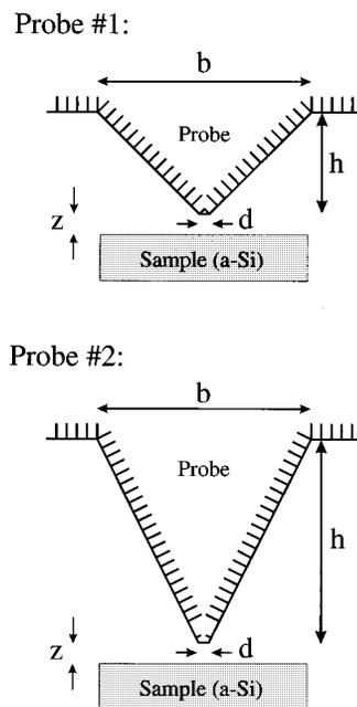
FIG. 4. Geometry of the probe-sample system considered in the numerical simulations. Probe No. 1:  $b = 2 \mu\text{m}$ ,  $h = 1 \mu\text{m}$ , and  $d = 20$  nm. Probe No. 2:  $b = 2 \mu\text{m}$ ,  $h = 2 \mu\text{m}$ , and  $d = 20$  nm. The illumination wavelength is 457.9 nm. The refractive index of the sample is estimated to be 4.35. The probe-to-sample distance is 5 nm, i.e.,  $z = 5$  nm.
