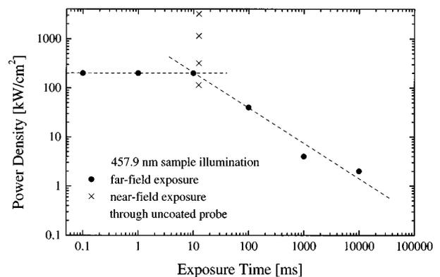
FIG. 10. Minimum power density, at  $\lambda=457.9$  nm, required for the formation of an oxide layer sufficient for KOH etching (dashed line). The four crosses indicate the working points for SNOM with uncoated fiber probes.
