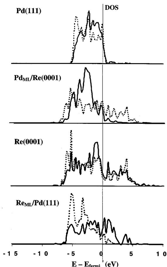
FIG. 2. Electronic density of states (DOS) projected to the  $d$  band of bare slabs. Solid lines indicate DOS projected to  $d$  band of the topmost layer. Dotted lines correspond to  $d$  band of the second metal layer.
