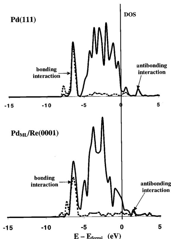
FIG. 5. Projected DOS for hydrogen chemisorbed on Pd(111) and Pd<sub>ML</sub>/Re(0001) systems. Solid lines correspond to DOS projected to surface metal  $d$  band. Dotted lines correspond to DOS projected to the H  $1s$  state.
