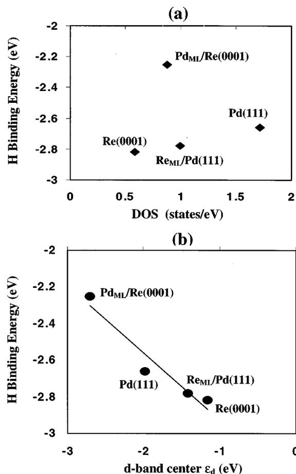
FIG. 7. (a) Binding energy of atomic hydrogen at the threefold fcc site as a function of the DOS at the Fermi level for the bare surfaces. (b) Binding energy of atomic hydrogen as a function of the  $d$ -band center for the clean metal surfaces (Hammer-Nørskov model).  $d$ -band centers are relative to the Fermi energy.
