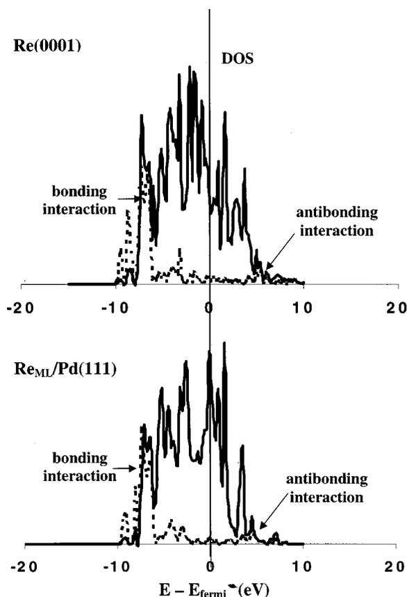
FIG. 6. Projected DOS for hydrogen chemisorbed on Re(0001) and  $\text{Re}_{\text{ML}}/\text{Pd}(111)$  systems. Solid lines correspond to DOS projected to surface metal  $d$  band. Dotted lines correspond to DOS projected to the H  $1s$  state.
