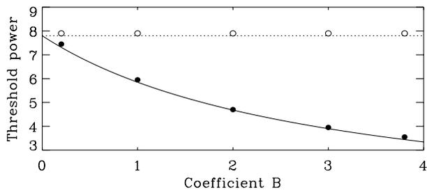
FIG. 1. Collapse threshold power  $2\mathcal{P}_c^B$  versus  $B$  for  $u_1(\vec{r}, 0) = u_2(\vec{r}, 0)$  with  $A = 2$  (solid line). The dotted line represents  $2\mathcal{P}_c^0$ . The black and white marked points indicate the numerically calculated collapse thresholds for  $\beta = 0$  and  $\beta = 20$ , respectively.
