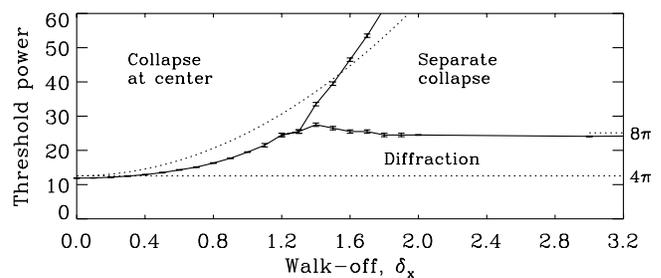
FIG. 2. Collapse threshold versus  $\delta \equiv \delta_x$  ( $\delta_y = 0$ ) for equal waves with  $A = 1$ . The solid curve, where error bars have been specified for the sake of accuracy, represents the numerical result for  $P_1 = P_2$  and  $\Delta = 2$ . The dotted lines correspond to the analytical predictions  $\mathcal{P}_{\text{th}}(1 + \delta^2)$ ,  $8\pi$ , and  $\mathcal{P}_{\text{th}} = 4\pi$ .
