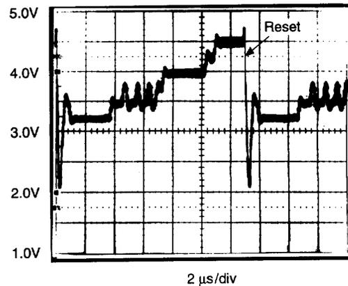
Fig. 7. Oscilloscope snap shot of adaptive supply scaling.
