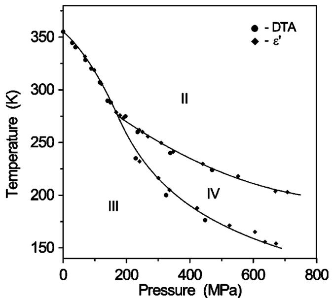
FIG. 5.  $p$ - $T$  phase diagram of  $G_2SnCl_4$ .
