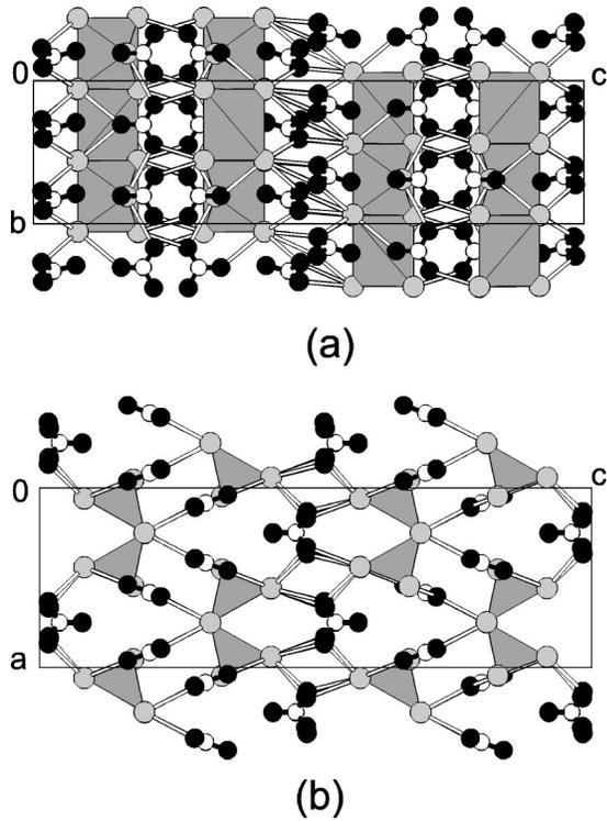
FIG. 3. The crystal structure of  $G_2SnCl_4$  at 293 K viewed (a) along the  $a$  axis and (b) the  $b$  axis. Sn is in the square pyramids having grey chlorides at the corners. Guanidinium ions are shown with white carbon and black nitrogen atoms, the hydrogen atoms are omitted for clarity. Hydrogen bonds are drawn open.
