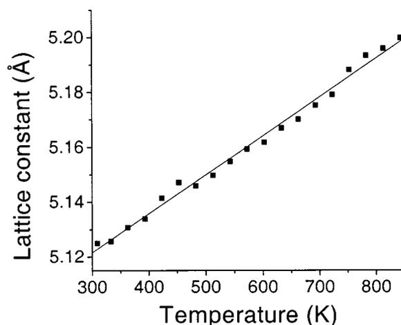
FIG. 3. Linear thermal expansion of as-solidified Cd<sub>83</sub>Ca<sub>17</sub> quasicrystals.
