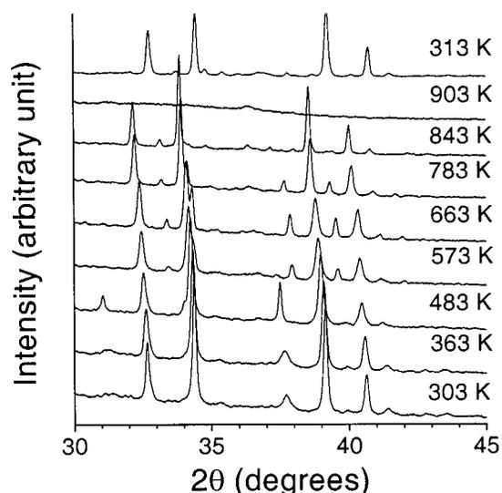
FIG. 2. *In situ* high-temperature x-ray powder diffraction patterns recorded with synchrotron radiation with wavelength 1.513 852 Å for the as-solidified Cd<sub>83</sub>Ca<sub>17</sub> alloy.
