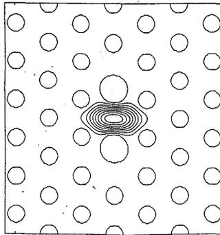
Fig. 1. High-birefringent PCF design. The birefringence arises due to the two enlarged air-holes near the center of the fiber, which breaks the 60 degrees symmetry. The field solution shown is for  $\frac{\Lambda_1}{\lambda} = 3$ , where the birefringence is  $5 \times 10^{-4}$
