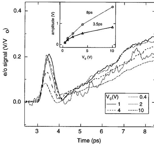
Fig. 5. E/o sampling data for different voltages on SI GaAs substrate. Pump wavelength is 760 nm and  $P_{opt} = 20$  mW. Signals are normalized to the applied voltage. The inset shows the amplitude dependence for the fast (at 3.5 ps) and slow (at 8 ps) component.
