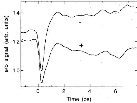
Fig. 9. Dependence on probe position. Pump beam is slightly overlapping the positive electrode. Substrate material is InP, electrode spacing is 10  $\mu\text{m}$ , and pump beam diameter is 3  $\mu\text{m}$ . The offset due to the modulated bias is not subtracted and the sign is not reversed.
