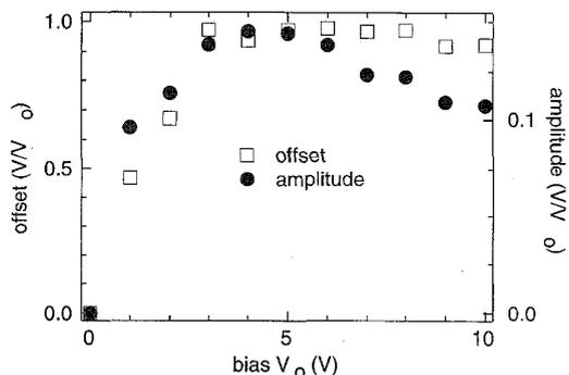
Fig. 13. Offset and amplitude of the fast component (at 200 fs) of the  $e/o$  signal in Fig. 12. An offset of  $V/V_0 = 1$  indicates that the field is modulated between 0 and the average field. For small voltages, the voltage drop at the contacts reduces the signal.
