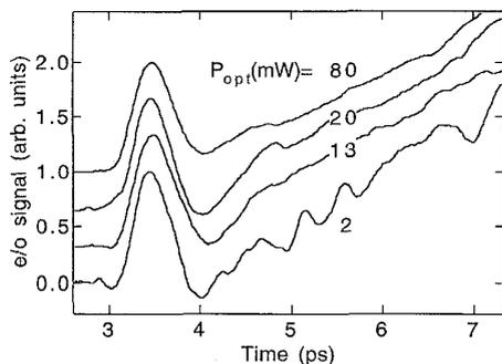
Fig. 3. Dependence on pump power. Amplitudes are normalized to the peak at 3.5 ps, and different offsets are added to the curves. The measurement is taken with a Ti : sapphire laser at 760 nm,  $V_0 = 10$  V.
