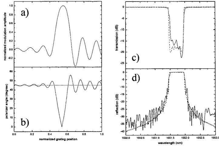
Figure 2. (a) Normalized modulation amplitude and (b) corresponding polarizer angle for a 99% reflectivity grating. The dashed line at  $\alpha=45^\circ$  marks the cross over between segments of the grating with different phase. Transmission (c) and reflection (d) spectra for a 23mm long FBG written in a deuterium loaded HNLf fiber.
