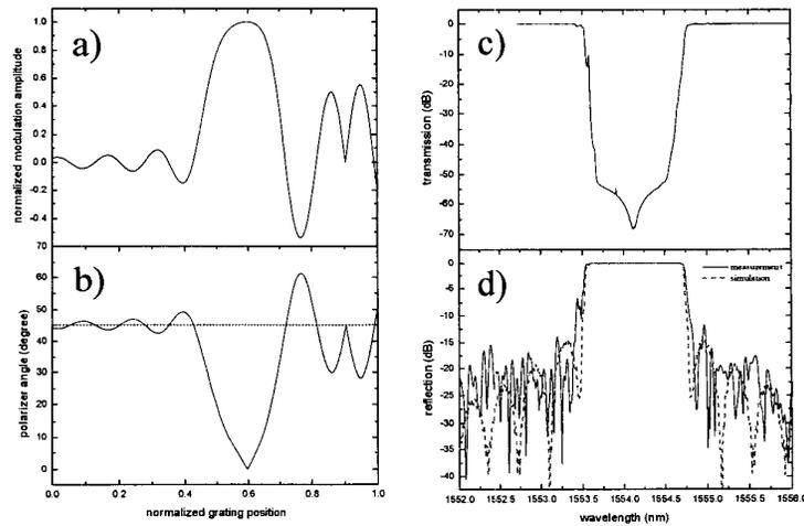
Figure 3. (a) Normalized modulation amplitude and (b) corresponding polarizer angle. The dashed line at  $\alpha=45^\circ$  marks the cross over between segments of the grating with different phase. Transmission (a) and reflection (b) spectra for a 23mm long FBG written in a deuterium loaded HNLf fiber.
