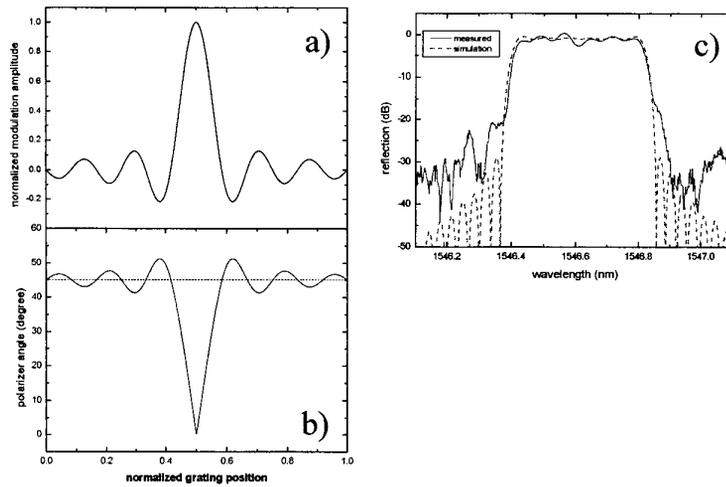
Figure 1. (a) Normalized modulation amplitude and (b) corresponding polarizer angle for a Sinc grating. The dashed line at  $\alpha=45^\circ$  marks the cross over between segments of the grating with different phase. Reflection spectrum (c) for a 23 mm long weak Sinc-grating written in deuterium loaded TW-fiber.
