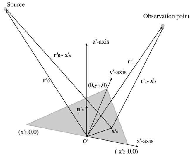
FIG. 2. Geometry applied for field integration over the surface of a triangular facet.
