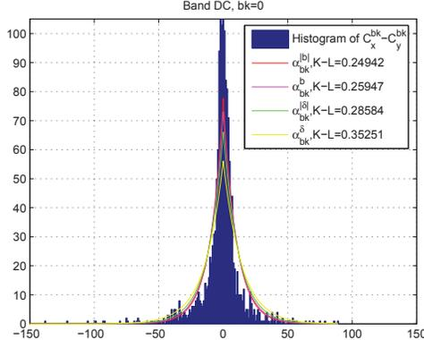
**Fig. 2.** Histogram of the actual residual  $C_{R_{XY}}^0 = C_{X_{2i}}^0 - C_{Y_{2i}}^0$  and the estimated distributions with different estimators (DC coefficients, frame 22 of Foreman). Kullback-Leibler distances (KL) are calculated to compare the distance between the true distribution and modeling distribution.
