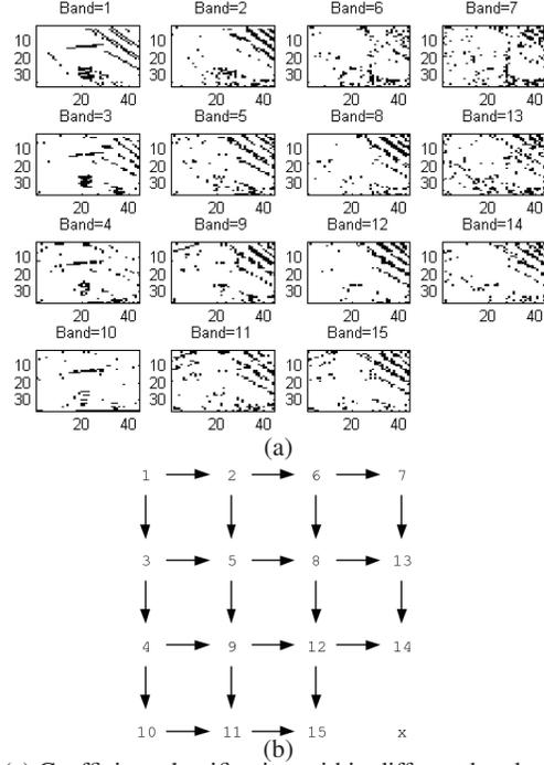
**Fig. 3.** (a) Coefficient classification within different bands tested on the actual residual  $C_{R_{XY}}^{b_k}$  (Frame 22 of Foreman). (b) The classification estimation from lower frequency band to higher frequency band
