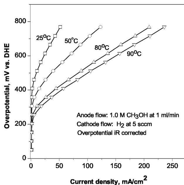
**Figure 10.** Methanol oxidation overpotential vs current density at different temperatures. Anode:  $\sim 1.5 \text{ mg/cm}^2$  Pt1Ru1. Cathode:  $\sim 2 \text{ mg/cm}^2$  20% Pt/Vulcan carbon (E-TEK).
