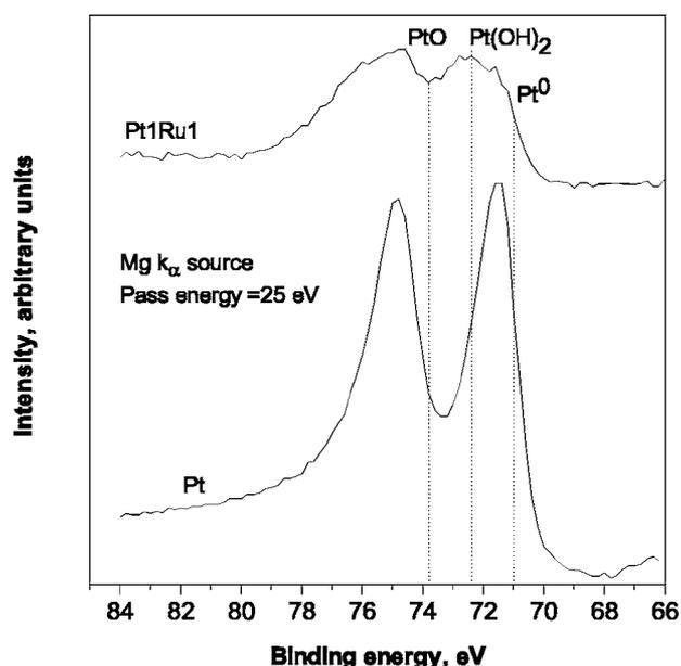
**Figure 6.** The XPS spectra for the Pt 4f core region of Pt and Pt1Ru1 catalyst layers on GDL. The vertical lines are the literature reported values for the binding energies of different oxidation states of Pt.
