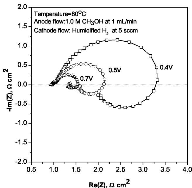
**Figure 9.** Nyquist plots showing the effect of anode potential vs DHE on the methanol oxidation kinetics at the DMFC anode as determined by impedance spectroscopy. Anode:  $\sim 1.5 \text{ mg/cm}^2$  Pt1Ru1. Cathode:  $\sim 2 \text{ mg/cm}^2$  20% Pt/Vulcan carbon (E-TEK).
