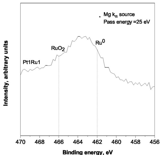
**Figure 7.** The XPS spectra for Ru 3p<sub>3/2</sub> core region of Pt1Ru1 catalyst layer on GDL. The vertical lines are the values reported in literature for the binding energies of different oxidation states of Ru.
