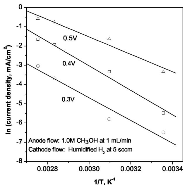
Figure 12. Arrhenius plot at different overpotentials. Anode:  $\sim 1.5$  mg/cm<sup>2</sup> Pt1Ru1. Cathode:  $\sim 2$  mg/cm<sup>2</sup> 20% Pt/Vulcan carbon (E-TEK).
