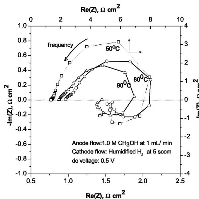
**Figure 11.** Nyquist plots showing the effect of temperature on methanol oxidation kinetics as determined by impedance spectroscopy at a dc voltage of  $0.5 \text{ V}$  vs DHE. Anode:  $\sim 1.5 \text{ mg/cm}^2$  Pt1Ru1. Cathode:  $\sim 2 \text{ mg/cm}^2$  20% Pt/Vulcan carbon (E-TEK).
