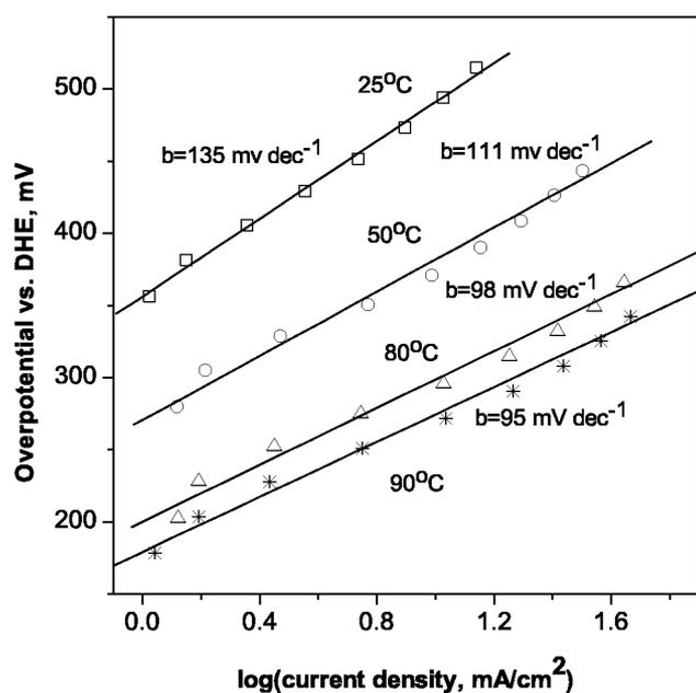
**Figure 8.** Overpotential vs  $\log(i)$  at different temperatures for methanol oxidation: 1 mL/min, 1.0 M  $\text{CH}_3\text{OH}$  at the anode, and 5 mL/min humidified  $\text{H}_2$  at the cathode. Anode:  $\sim 1.5 \text{ mg/cm}^2$  Pt1Ru1. Cathode:  $\sim 2 \text{ mg/cm}^2$  20% Pt/Vulcan carbon (E-TEK).
